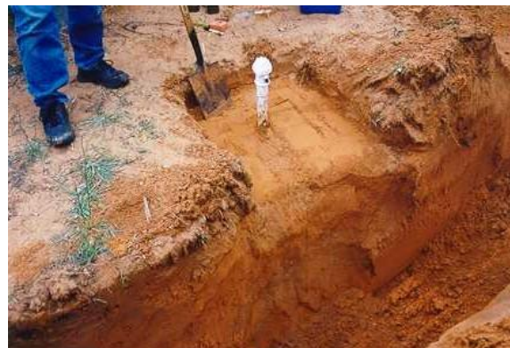
Photo 3. Digging platform for sampling
