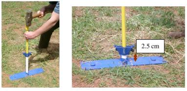
**Note**: This clearance height is important. If you hammer the probe in too far you will not be able to lift the stabilization plate off the long stabilization plate pins.
