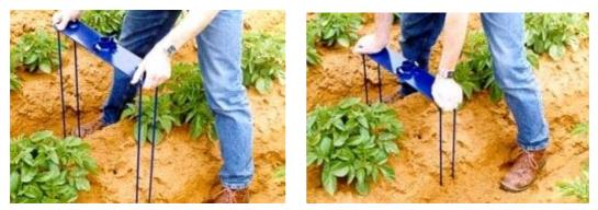
4. Using a *sledgehammer* alternately beat the *stabilization plate* at the points provided to force it closer to the ground. Do not beat continuously on any one side in advance of the other. The aim is to achieve a situation where the pins are near parallel in the ground.
