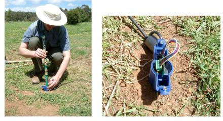
2. Pull the excess cable back through the cable gland. The outer sheath of the cable should be trimmed back as far as the point where the cable enters the inside of the top cap. Apply silicone around the wires of the cable at the end of the outer sheath, to prevent moisture from traveling along the cable into the inside of the top cap.
