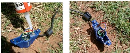
3. Ensure that the sealing gasket on the top cap is **clean**, in and positioned correctly, and replace the *lid* of the *top cap*. Tighten the screws evenly completely to ensure an effective seal.
