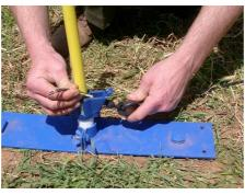
6. Remove the stabilization plate wing nuts.
