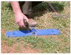
6. If the soil is dry, add a small quantity of water into the hole using a squirt bottle.
