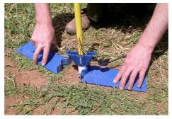
8. Continue inserting the probe into the ground with **gentle** blows of the *sledgehammer* using the *dolly*, until the base of the *top cap* is level with the ground. This will place the top *sensor* at 10 cm (3.9 inches) below the ground surface. Remove the dolly.
