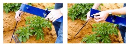
2. Place the assembled *stabilization plate* on the ground directly above the required position of the *probe*.
