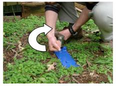
4. Carefully lift the *soil sampler* directly out of the ground. To remove the soil collected in the *soil sampler*, simply beat on its side with the hand or foot. The design is such that the soil core taken is slightly compressed, and of a lesser internal diameter than the *soil sampler* itself. In heavier textures, the *soil sampler* cleaning tool is used to clear the *soil sampler*. The extracted soil should be deposited away from the *probe* site.
