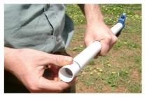
2. Remove the lid of the *top cap* and extract the probe electronics. Place these safely to one side on a clean, dry surface such as a tarpaulin.
