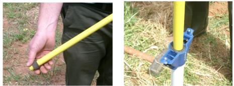
4. Continue inserting the *probe* by hammering on the insertion dolly with a *sledgehammer* until there is a 2.5 cm (1 inch) gap between the base of the top cap and the edge of the *stabilization plate* tube guide.
