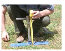
Warning: Do not compress the soil around the insertion site such that normal water infiltration is inhibited 3. Turn the soil *sampler* one single complete rotation clockwise.
