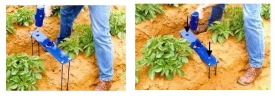
5. The *stabilization plate* should be firm to the ground without causing significant soil compression.
