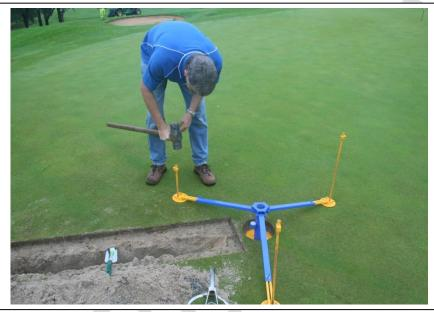
Insert pins by hammering to full depth.
