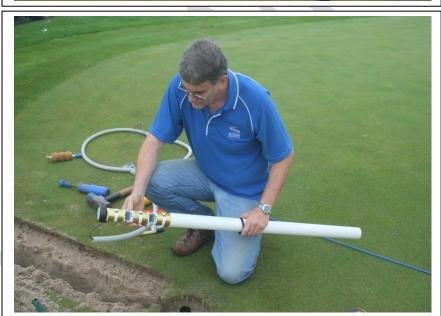
Attach a fresh silica gel bag with a cable tie as shown.
