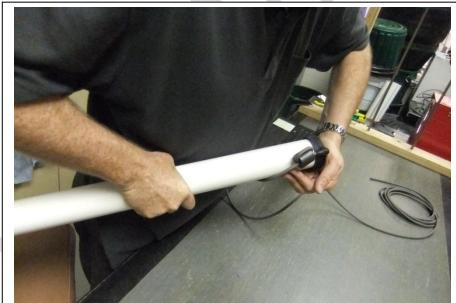
Hold the access tube such that nothing approaches in close proximity of any of the sensors (allow 14cm clear around it).
