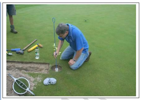
Inspect the inside of the access tube with a light on a string to confirm that it is clean.
