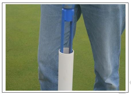
Insert 47 mm Auger into access tube and auger out soil to a depth no greater than 10 cm ahead of the access tube.
