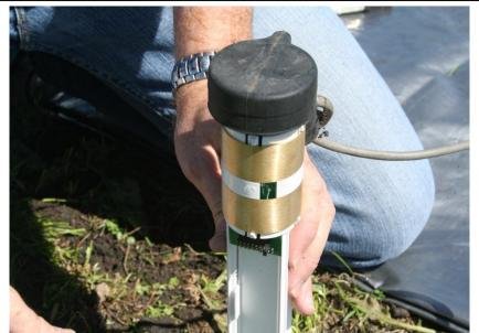
Plug sensor back into probe rod.
