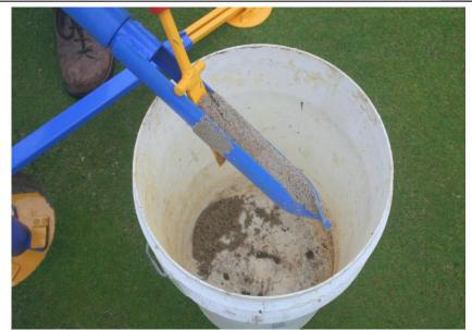
Remove auger from the access tube and clean out soil into a bucket to maintain a clean installation site.
