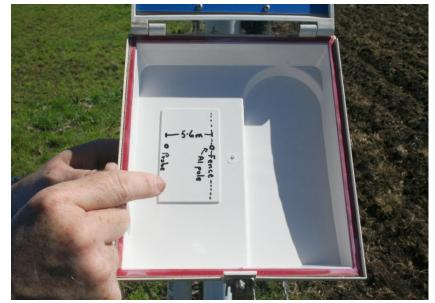
Ensure there is a drawing inside the DTU box indicating the distance and direction of the probe location in relation to the DTU pole. This will allow easy location of the probe at the next service call.
