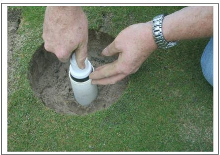
Tighten the bottom stopper near the top of the access tube until it is firm.
