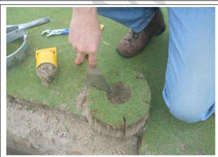
Re-insert the sod around the installed Flat Cap probe.
