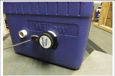
The top sensor cannot be normalized in the Normalization Container as there is a volume of air around it.
