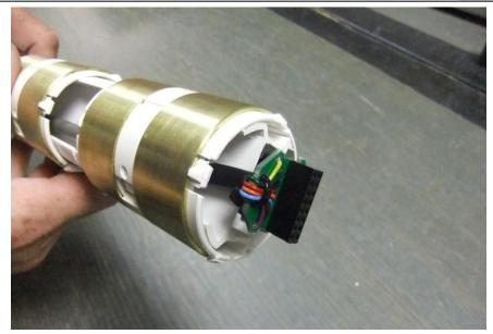
Pull the Internal Probe Cable tight.
