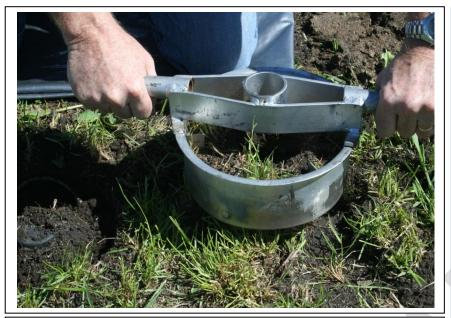
Carefully lift large Turf Cutter with the soil and set aside.
