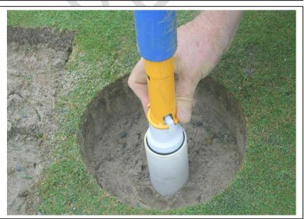
Fit bung tightening tool to bung.
