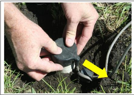
Apply firm pressure with both hands to re-seat Flat Cap onto the access tube.
