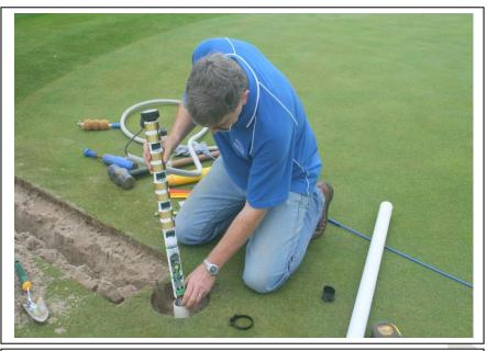
Carefully insert the probe electronics into the installed access tube.
