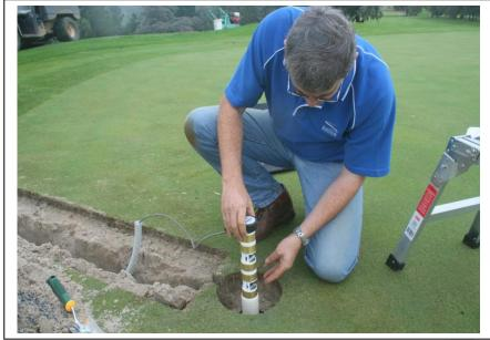
Remove probe again from access tube for final communication Test Upload.
