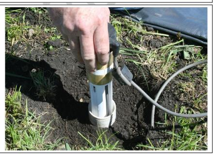
Gently push the probe back into access tube.
