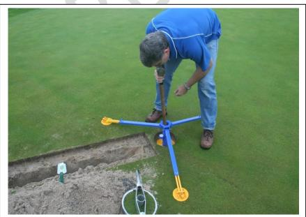
Loosen tripod thumb screws and insert handle of sledge hammer into tripod. Level the tripod by leaning on the hammer handle until the levelling bubble is centred. The tripod levelling bubble is centred enabling a straight auguring process.
