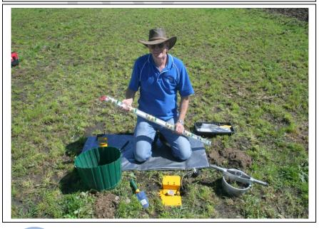
The probe can now be completely removed from the access tube and inspected.
