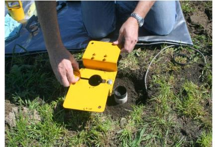
Remove Clamping Plate.
