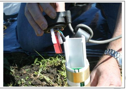
Remove Flat Cap from probe rod.
