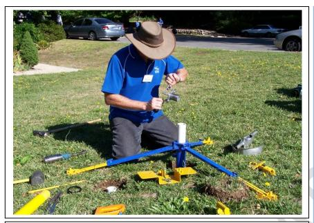
If you need to cut the top of the access tube off for any reason, it can be re-grooved in the field using the Groove Tool.
