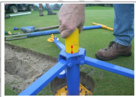
Remove the tripod pins using the Tommy Bars.
