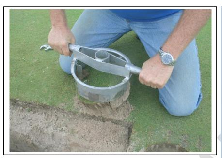
Remove the sod from the large Turf Cutter.
