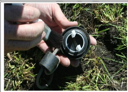
For hard to remove soil particles or stones use a screw driver. Be careful not to scratch any of the rubber ridges.
