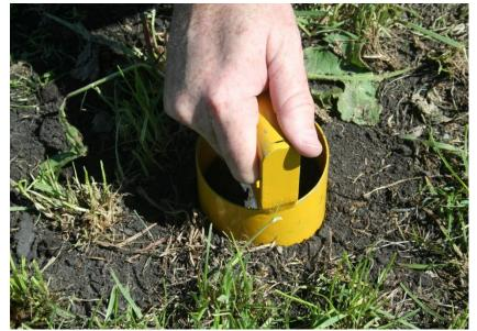
Push in small Turf Cutter with a rotating motion.
