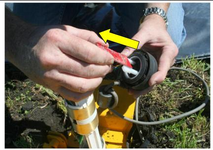
Unplug Flat Cap sensor board from Top Cap Assembly.
