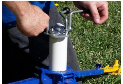
The access tube can be "squared off" by applying downward pressure and rotating the tool clockwise. Then position the tool at the second stop (engaging the spring lever).
