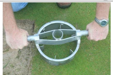
Place the large Turf cutter on the spot where the probe is to be installed.
