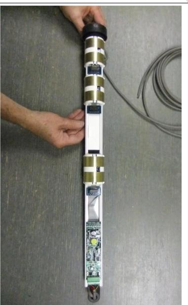
The completed Flat Cap probe.
