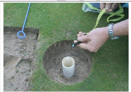
Insert Bottom Stopper into access tube.
