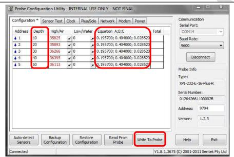
Set the sensor depths and calibration coefficients. Use the default calibration coefficients if you do not have site-specific data.
