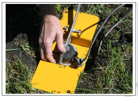
Place Cap Removal Pliers between the pins on the Clamping Tool and around Flat Cap.
