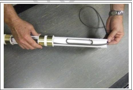
Make a loop in the cable, and squeeze it into position in the back of the probe rod.
