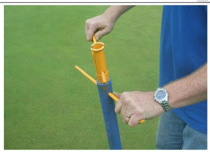
Attach and secure the bung tightening tool onto auger extension.
