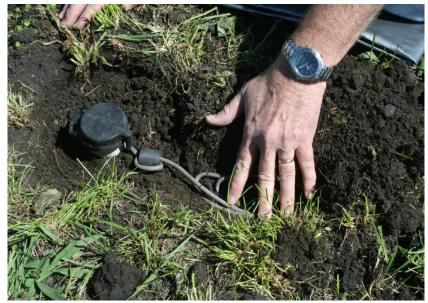
Loop the cable and position it about 20 cm away from the probe.
