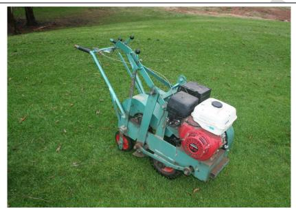
Use a sod cutter to cut sods from the DTU position to Flat Cap probe location and place to one site.
