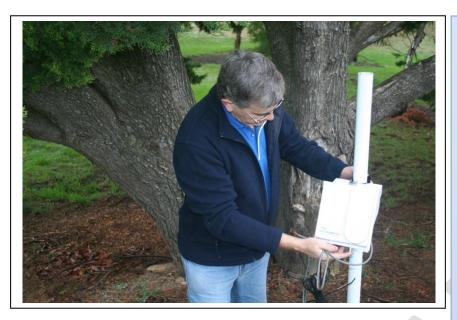
Select position of Sentek Data Transmission Unit (DTU) and Flat Cap probe location.
