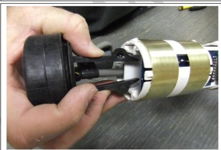
The sensor has been slid down to show the correct position of the Flat Cap clip feet fully engaged.
