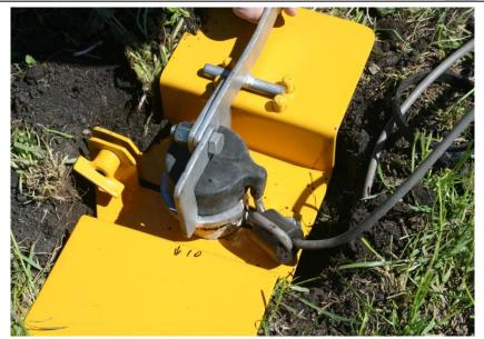
Push down the handle of the Cap Removal Pliers to separate Flat Cap from access tube.
