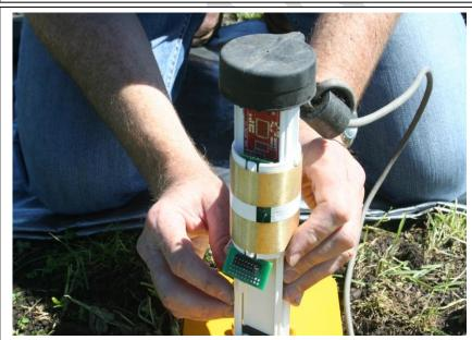
Push in clips of Top Cap Assembly to release Flat Cap from probe rod.
