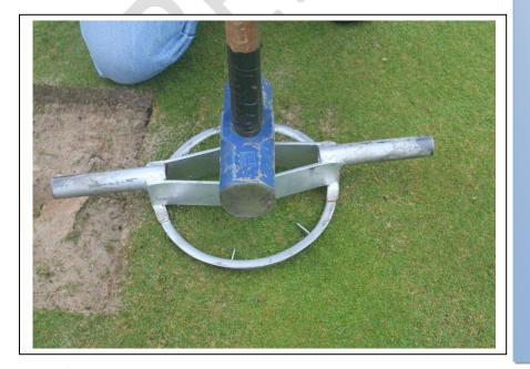
Use the sledge hammer to insert the Turf Cutter into the grass.
