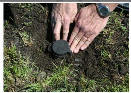
Position the large Turf Cutter with the grass sod set aside previously over the Flat Cap and gently push out the circular grass sod.
