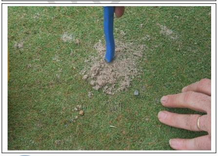
Repair tripod pin holes with soil.
