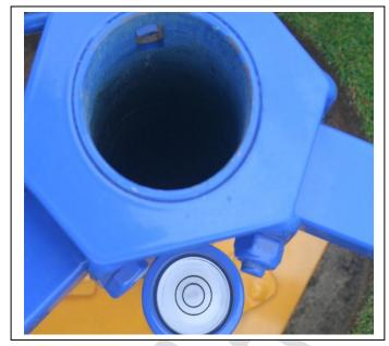
Use the metal Cutting Edge to remove the sharp internal edge of the access tube.
