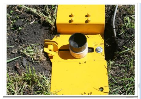
Protect the top of the access tube with a plug to prevent dirt falling inside it.
