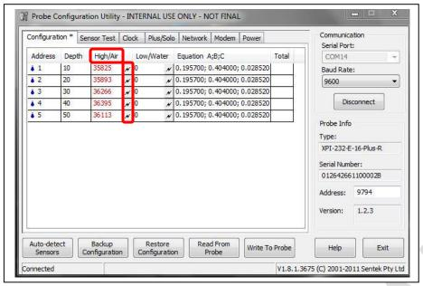
Set the Air Counts using the Probe Configurator software. Click individual sensor settings or column heading to set all sensors.
