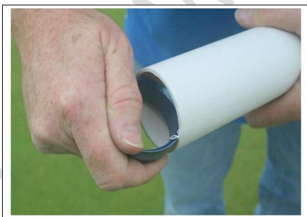
Place Cutting Edge into access tube and gently tap it on a hard surface to fully insert it.
