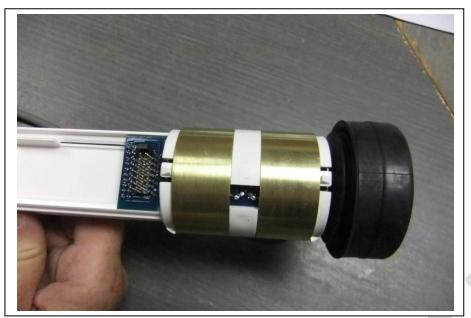
The fully attached Flat Cap with the top sensor in the correct position.
