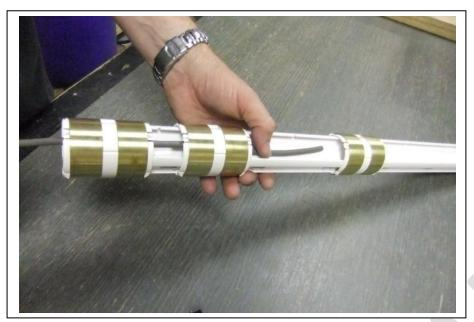
Thread the Internal Probe Cable through the sensors from top to bottom along the back of the probe rod.
