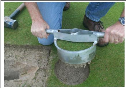
Set the sod aside with most of its root system intact.
