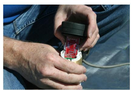
Now push Top Cap Assembly back onto the probe rod until the clips audibly click in and are fully seated.
