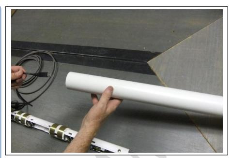
Seal the Flat Cap onto the top of the access tube.
