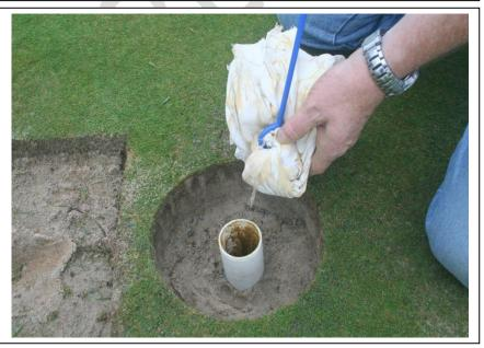
Insert rag tool into the access tube and push down.
