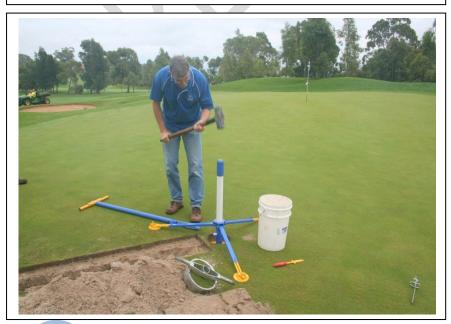
Alternately use the auger and sledge hammer to remove the soil just ahead of the Cutting Edge.
