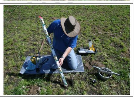
Reinsert serviced probe into the access tube.
