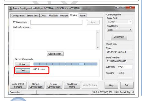
Perform a Test upload to ensure that communications are all working. The message "040 Success" should be returned. Replace Flat Cap probe into access tube and use firm downward pressure until the Flat Cap audibly "snaps" into place.
