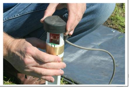
Now slide top sensor back into position and click into probe rod.
