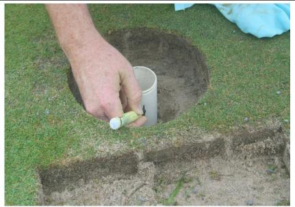
Protect against entry of dirt into the access tube with a temporary plastic black cap.
