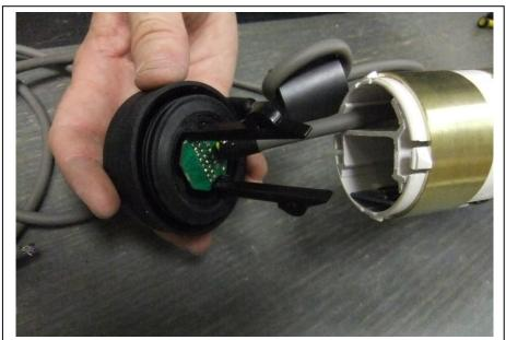
Squeeze the Flat Cap clip inwards and slide into place. An audible "click" occurs when the clip is fully engaged. A gentle twist may help in this.
