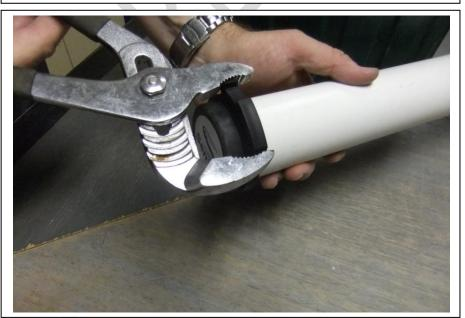
Remove the probe from the Normalization Container and insert it into an access tube. The access tube can be one prepared with a groove or not. Tighten the Flat Cap onto the top of the access tube with a Herbie™ Clip.
