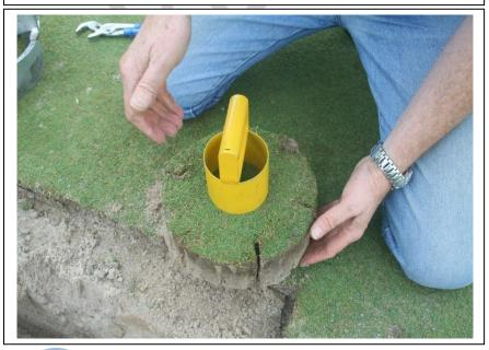
Position the small Turf Cutter in the centre of the sod and push it in.
