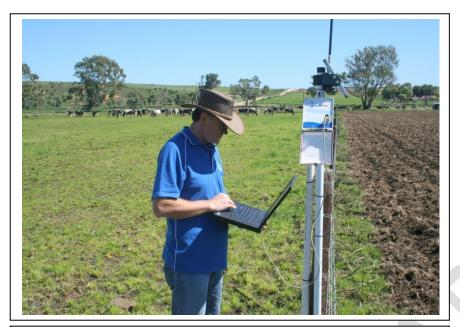
Plug your lap-top into the Data Transmission Unit (DTU) and check the sensor readings.
