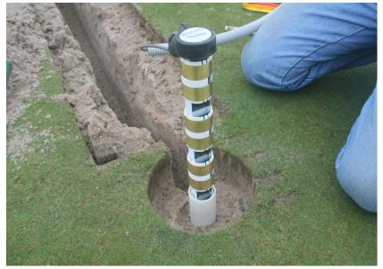
Align cable from Flat Cap probe with trench.
