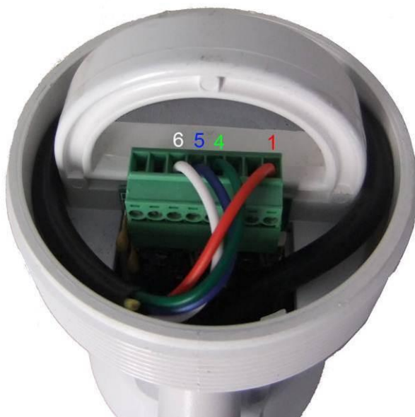
Figure 12 Probe sitting correctly in tube, showing correct wiring
