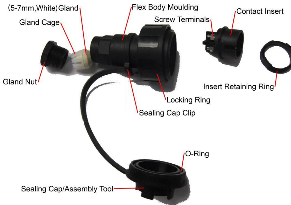
Figure 17 Sentek MULTI Probe Cable Connector
