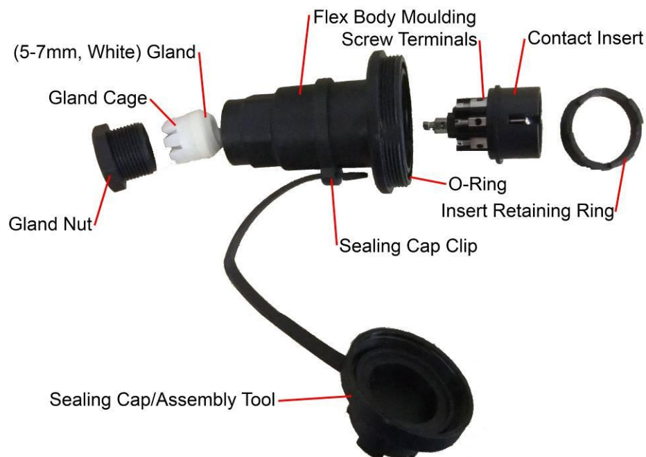
Figure 14 Sentek PLUS Probe Cable Connector (Probe cable side)
