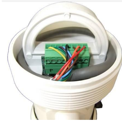
Figure 10 Probe sitting correctly in tube with connector in place
