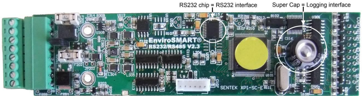
Figure 34 EnviroSCAN RS232 logging interface
