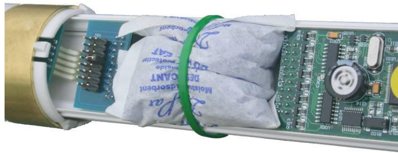
Figure 13 Silica gel bag placement
