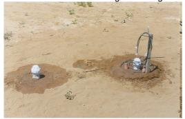
With all samplers installed, flood the area with around 10L of low EC water, and allow the water to infiltrate overnight. This will bed down the samplers, and ensure good contact between the soil and ceramic cup.
