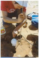
below the soil surface, pack a small amount of bentonite on top and poke slightly down the sides of the shaft, using the stick as before. Avoid placing bentonite too far down the shaft, as it will interfere with the operation of the ceramic cup.
