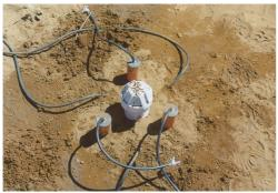
Stake the sample tubing from all the samplers in a vertical position, with the stopcocks at the top. This prevents soil or insects from contaminating the tubing.
