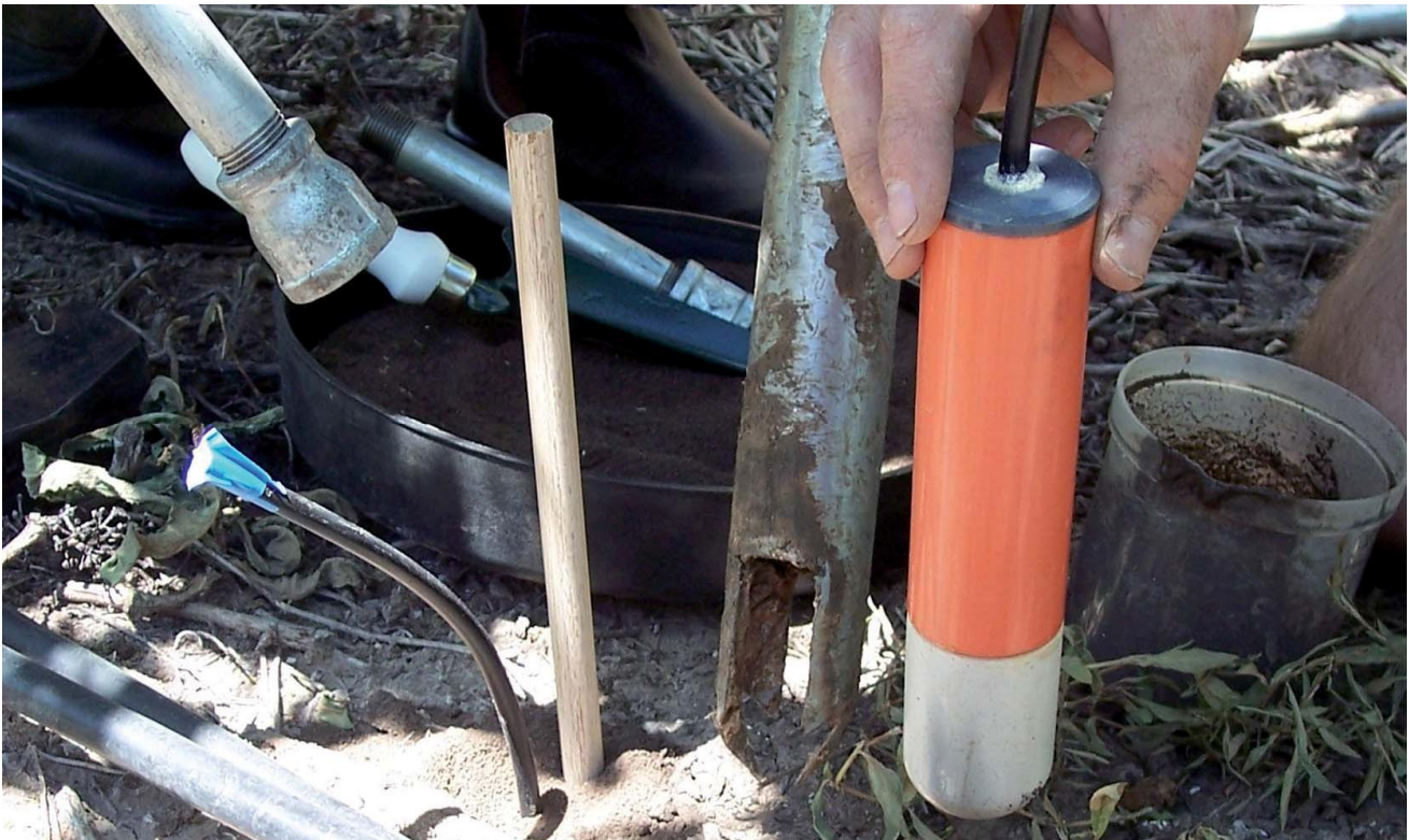
Figure 2. Equipment for installing the Sentek SoluSAMPLER™
