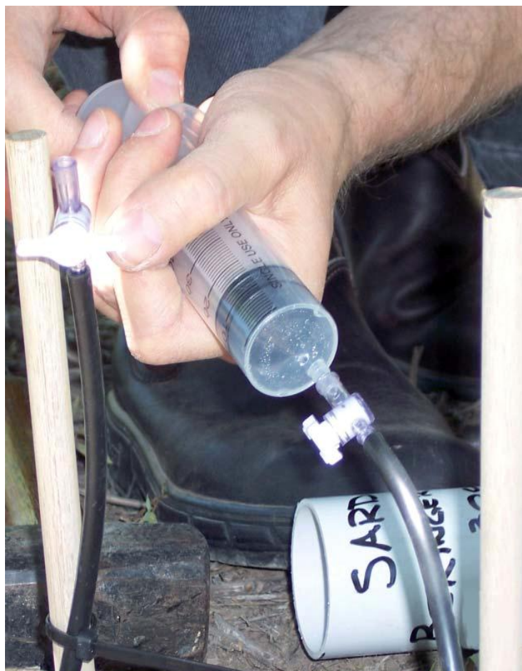
Figure 5. Drawing soil water
