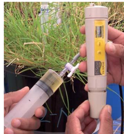
Figure 6 Extracting sample and reading the EC meter
